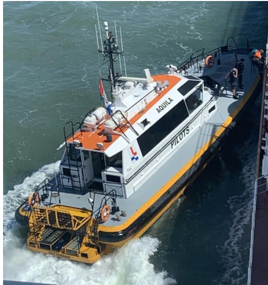
The AQUILA alongside a ship. Note the the massive MOB installation on her stern
