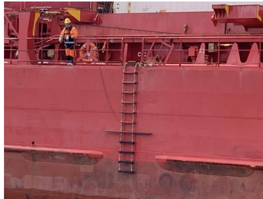
Fendering is clear in way of the pilot ladder (The gap should be 6m though!)
