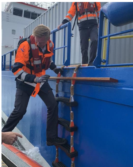
The minimum length of 1,5 m can barely be achieved on a small freeboard tanker
