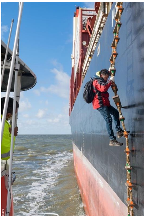
The spreader in action: preventing the twisting of the ladder during its use (Source: facebook group #dangerousladders)
