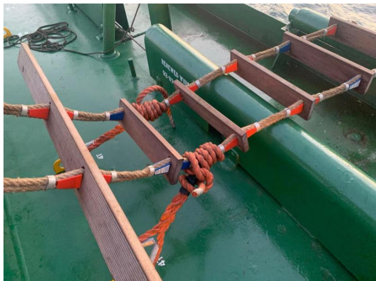
The rolling hitch knot used on a well rigged pilot-ladder arrangement. Observe the marked strong points on deck (SWL 4T) Pic: Cpt. Gary Clay,
