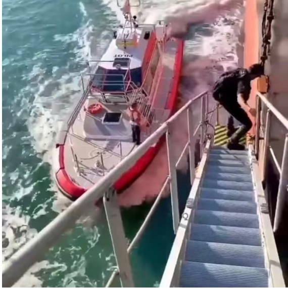
On the final step to the platform and onto the pilot ladder, the pilot has only one hand to hold himself if the inboard stanchion is not in place. (Source: Sea and Coast Magazine, via Facebook)
