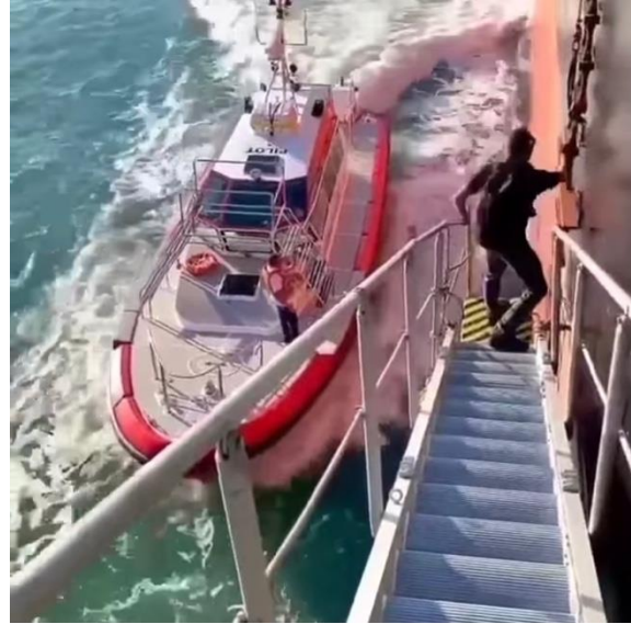
On the final step to the platform and onto the pilot ladder, the pilot has only one hand to hold himself if the inboard stanchion is not in place. (Source: Sea and Coast Magazine, via Facebook)
