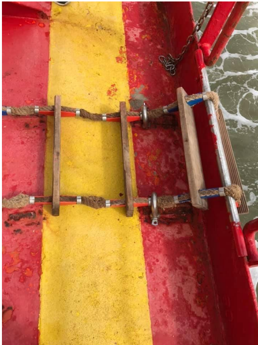
D-S Shackles: damaging to the chocks and steps
