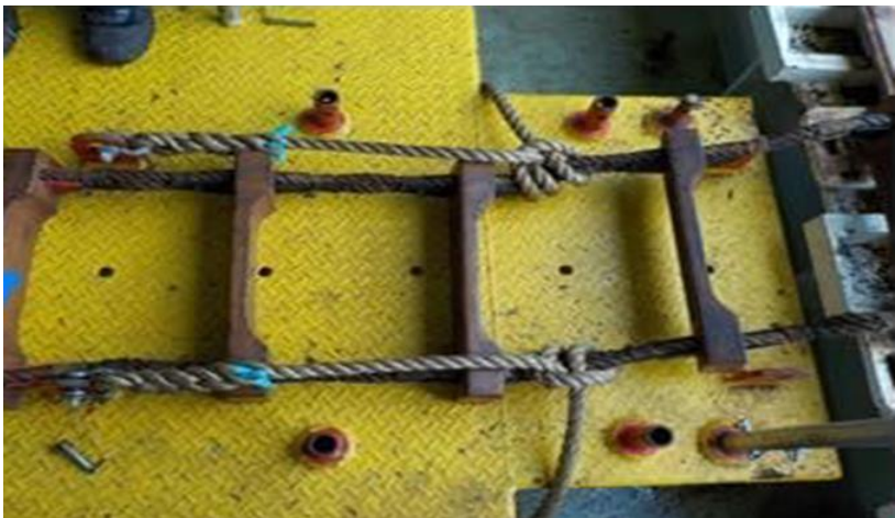
Figure 2 Side ropes need to be secured to a strong point, rope lashings, with a "Rolling Hitch".
