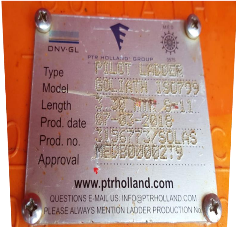
Figure 3 Example of a Plate from a major manufacture of Pilot ladders, PTR Holland Group. Note the Date of Manufacture and Product Number.
