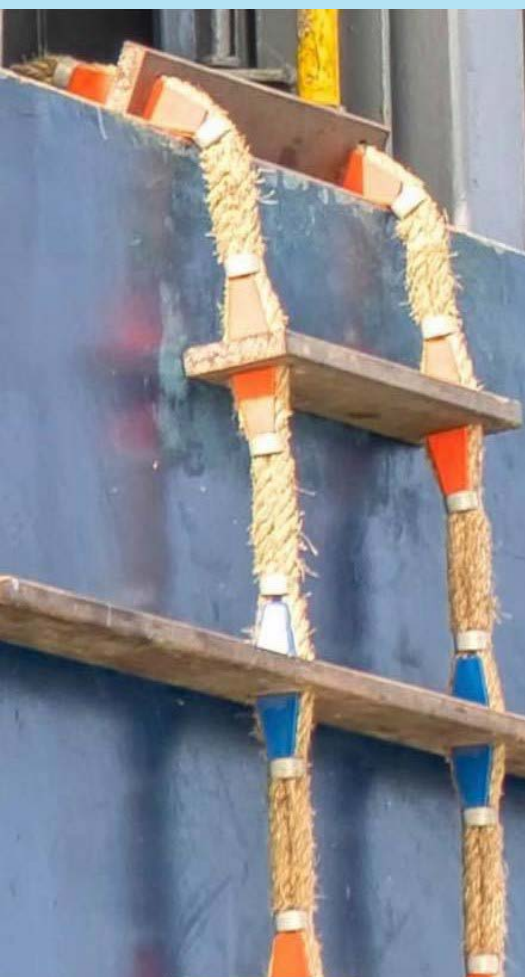
Pilot ladder over the side across a sharp edge.
