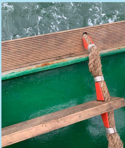
Wear and tear on the pilot ladder rope will occur at a faster rate if no sharp edge protection is in place.
