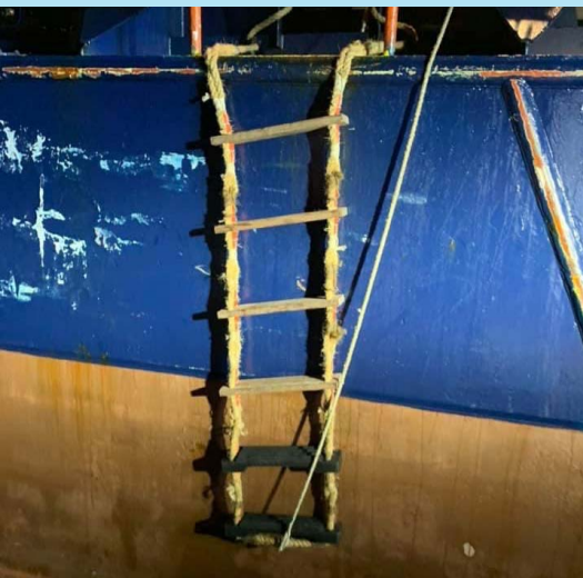
This ladder is not classified as a pilot ladder, since it has no spreaders and four rubber steps. The retrieval line is in the way of the steps.
