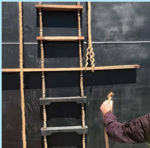
Frayed and broken man-rope.
