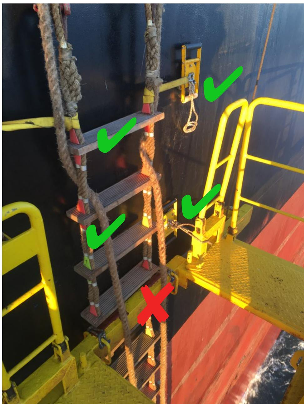
**#4 - Non-compliant example (this would be fully compliant if the railing and inboard beam were removed)**
