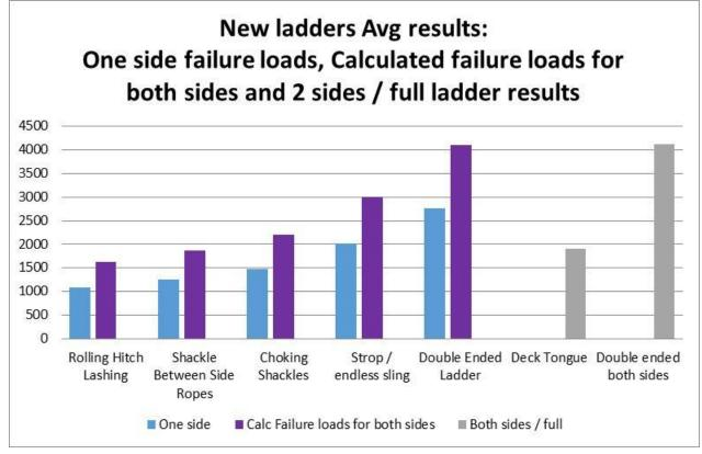
Sometimes the lashings using rolling hitches failed before the ladder did. All the other methods the side ropes failed before the securing gear did.
