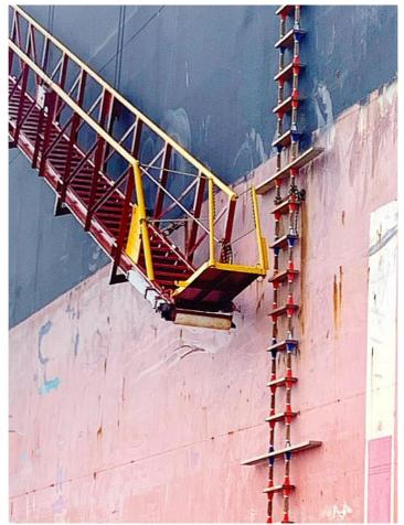
A well secured combination pilot ladder
