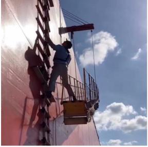
In the next picture (left), the pilot embarks a vessel using a combination ladder. The first thing he grabs when he steps off the pilot ladder onto the accommodation ladder is the inner stanchion. It is the closest to the pilot ladder and that's why it is very important for getting balance when stepping onto the platform.
