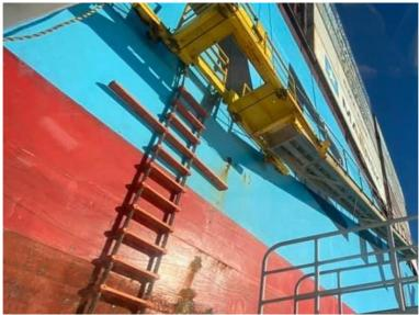
A non-compliant trapdoor arrangement: Pic: Marinelog article
