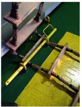
Steel Bar: damaging to the chocks and steps of the ladder
