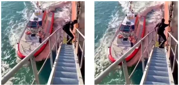
On the final step to the platform and onto the pilot ladder, the pilot has only one hand to hold himself if the inboard stanchion is not in place. (Source: Sea and Coast Magazine, via Facebook)
