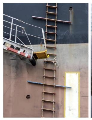
The above ladder was presented in December 2020, when the pilot boarded a vessel: Securing incorrect, Steps not straight, Inner stanchion is missing, coating or tape on the spreaders...
