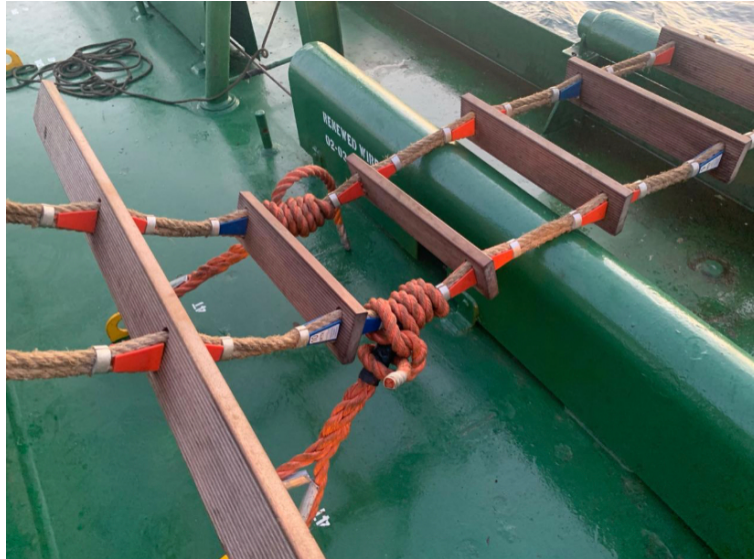
The rolling hitch knot used on a well rigged pilot-ladder arrangement. ( Ideally the securing ropes should be manila ) . Observe the marked strong points on deck (SWL 4T) Pic: Cpt. Gary Clay,
