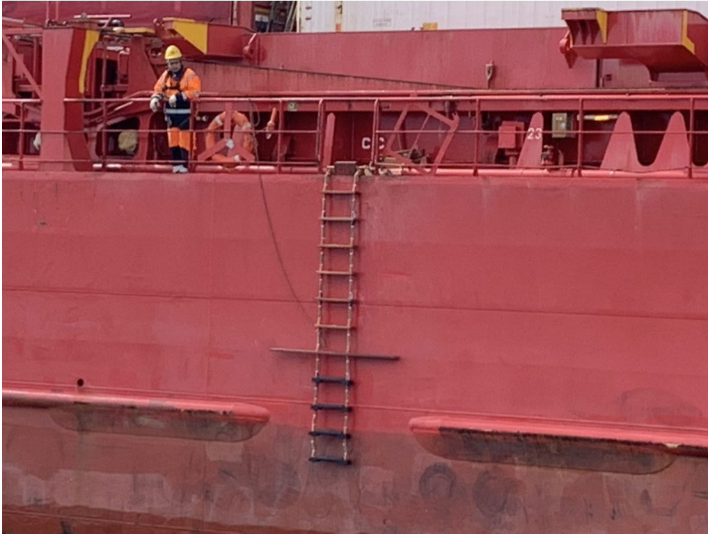
Fendering is clear in way of the pilotladder (The gap should be 6m!)
