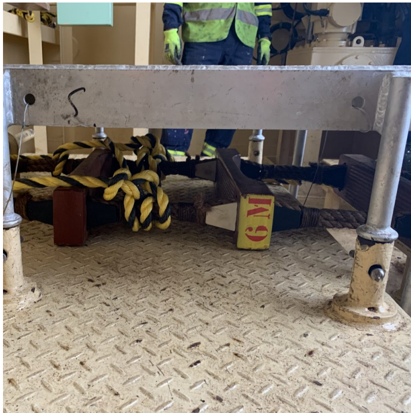
Pilot ladder from a winch, secured by rolling hitch knots.
